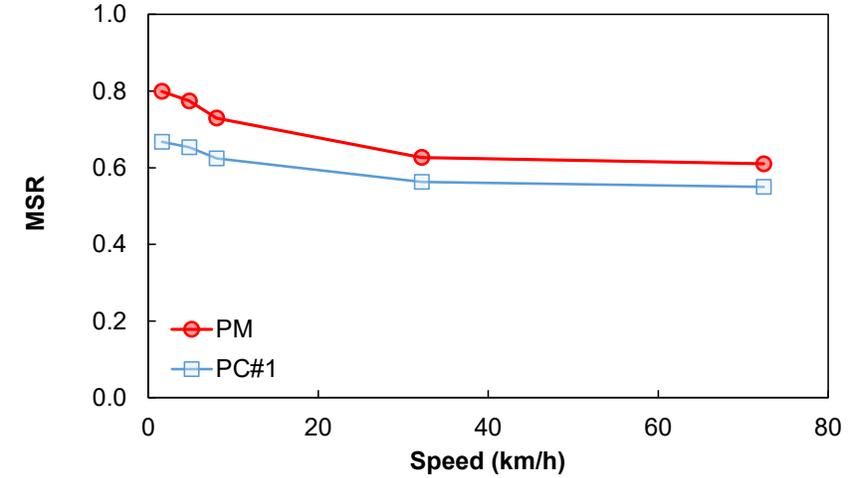
❑ The interlayer shear resistance is poorer when the vehicle speed is lower.
